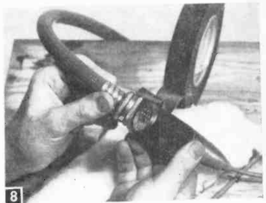
It's important that no outside sound reaches the pick-up mike. Cover the hose connection with a thin wrapping of medical cotton and tape. Then cover with a heavier layer of cotton, and again tape tightly. From funnel to microphone, there can be no sharp bends in the hose line.
