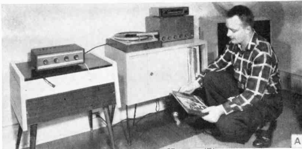
The reverb unit's pickup mike feeds through a separate amplifier and speaker. You can use this system with both monaural and stereo tapes or records.
