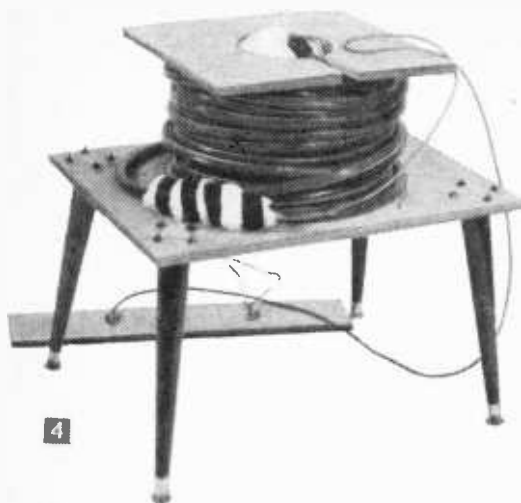
4 The core is one unit. The cabinet is a separate unit that fits over the top. You can adjust the legs shown for straight or angle mounting. Two jacks on the front panel connect to the monitor speaker and the pickup mike.
