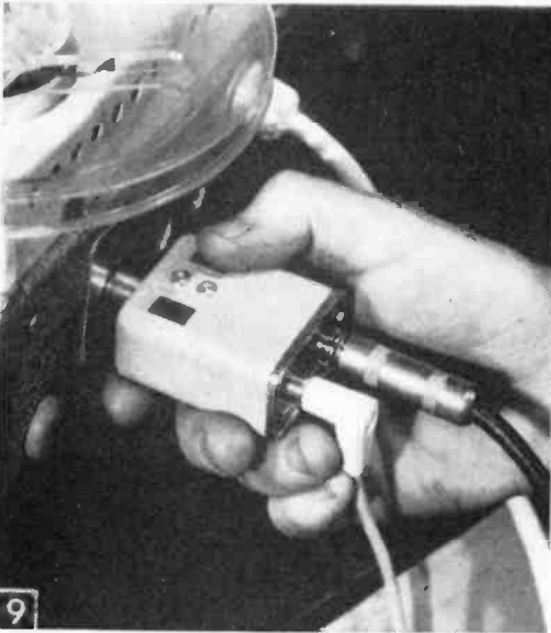
9 The Mini-Mix has two built-in volume controls that blend your input microphone lines. You can use it with the reverb system, as well as on your tape recorder.
