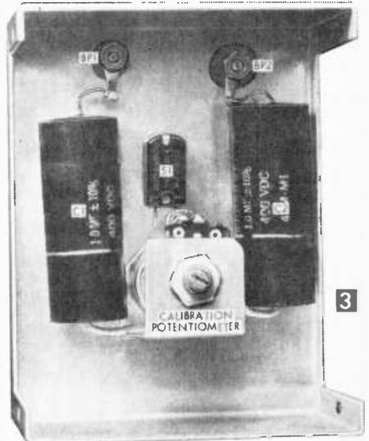
Back view of calibrator shows parts placement. Note the slotted shaft on the calibration potentiometer (R2).
